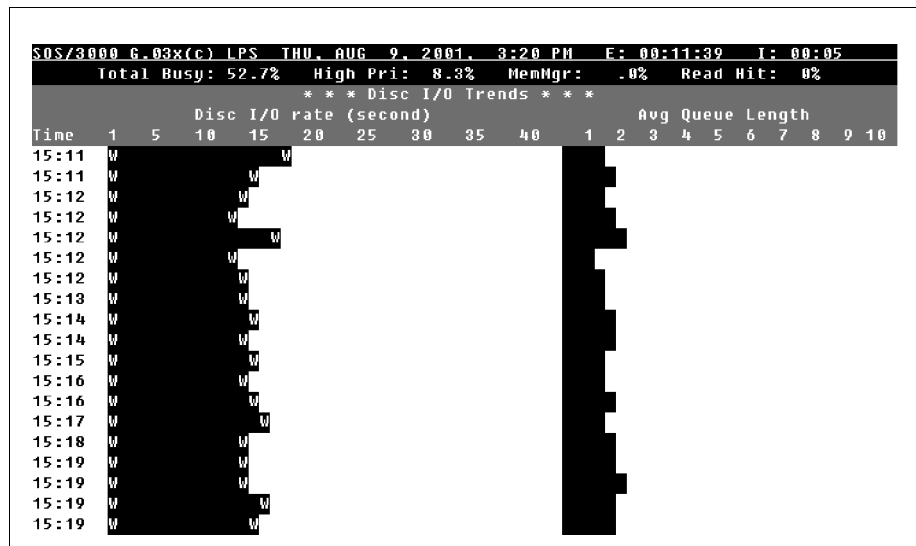
Figure 11.3 SOS Disc I/O Utilization Trends screen
